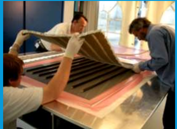
Embedded heat pipes mounting
