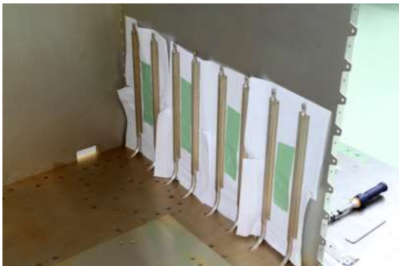
Under: Embedded and surfaced heat pipes on ACES
