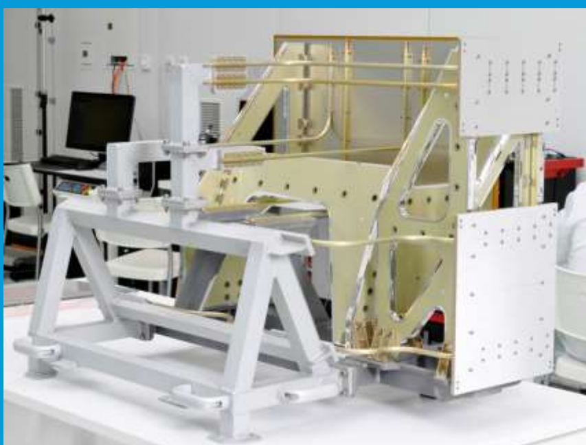
Above: Heat pipes on EUI OBS
