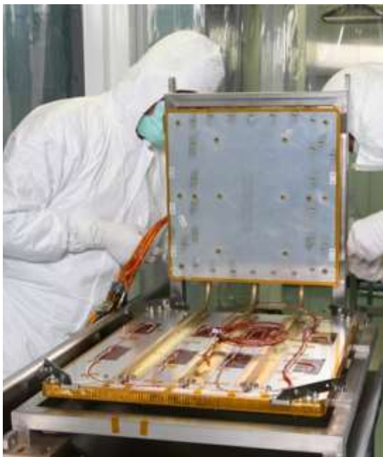
Above : Heat pipes on Sentinel-3 OLCI
