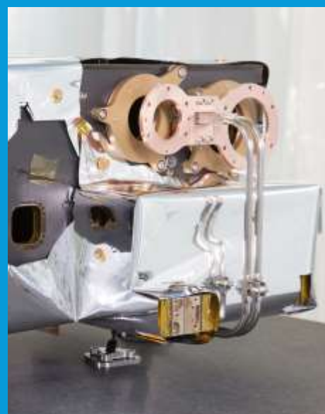
Above: Heat pipes on EUI OBS
